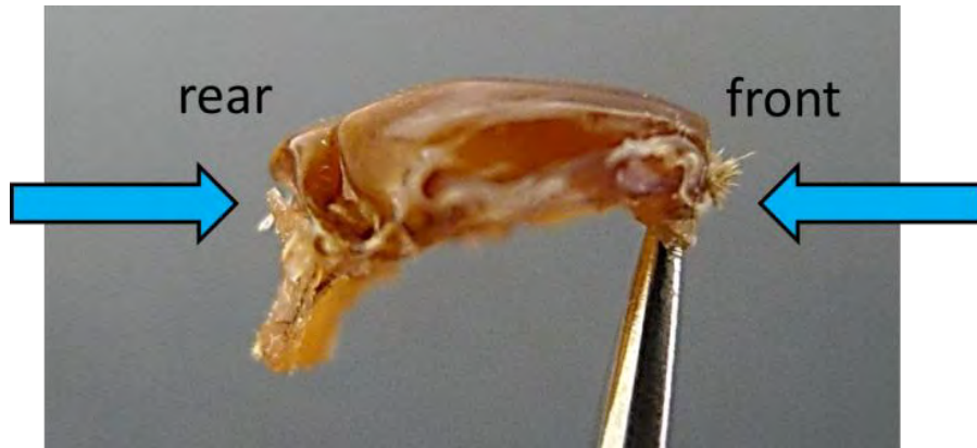
Figure 98 - Location of longitudinal compressive force simulating DLM contraction. This image shows only the tergum, but the entire thorax would be intact for this experiment. The head and abdomen must be removed for access to the load application points at the front and rear phragma.
