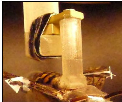
Figure 48 – Proof-of-concept phase of dynamic load experiment. Note paper scraps glued to wings for tracking wing angles. This practice was subsequently deemed unnecessary.
