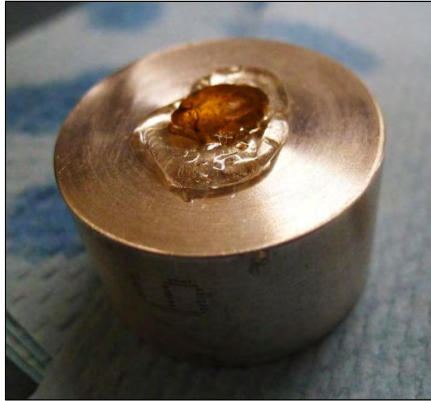
Figure 71 - Tergum mounted to puck with Crystalbond Hot Melt. The thermoplastic polymer completely fills and supports the cavity created by the removal of the flight muscles. The tergum is thin enough for light to pass through, giving the specimen the appearance of amber.
